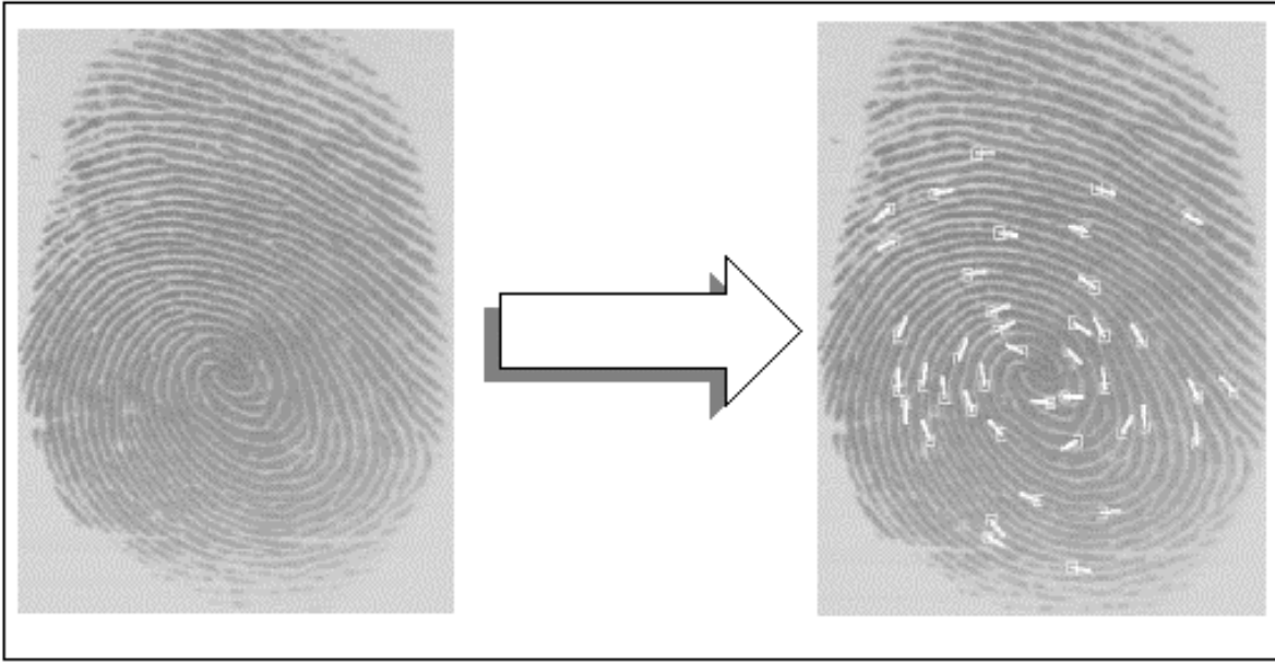
Figure 1. Finger Minutiae-Based Biometric Matching
